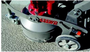
The Diamatic 435 WD machine weighs 115 kg with an operational speed of 720rpm
