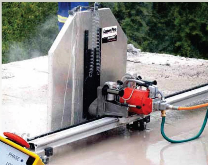
ABOVE: DP 75 H wall saw. FAR LEFT: Floor saw – 13 hp. LEFT: DP 75 H wall saw control unit.
