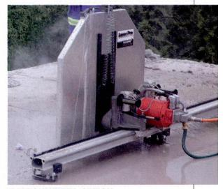
**ENVIRONMENTAL OPTION**The DP 75 H wall saw's electric design eliminates leaks that occur when many hydraulic wall saws are used
