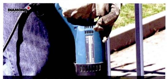
Diamond Products hand held water coring system requires an electric drill 700-1200 Watt with minimum 2000 RPM.
