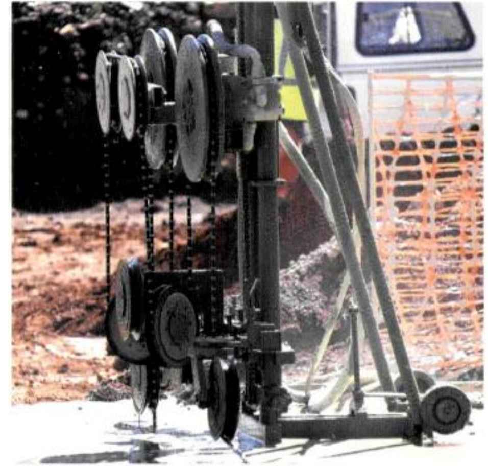
Versatile hydraulic diamond wire saw set up with Razor wire.
